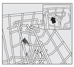
Pull the cup rack upwards and click it back into position at the required width.
